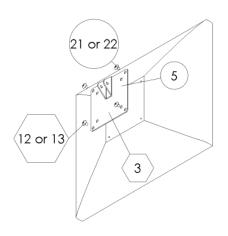
Step 5: Attaching the flat panel to the mounting plate
