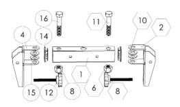
Step 3: Attaching the pivot bracket to the support tube
