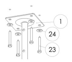
Step 2: Mounting the ceiling plate
