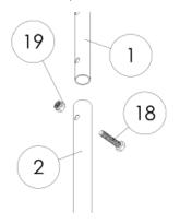
Step 7: Attaching the extension tube to the ceiling plate
