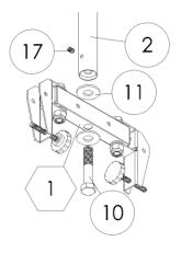
Step 4: Attaching the extension tube to the support tube
